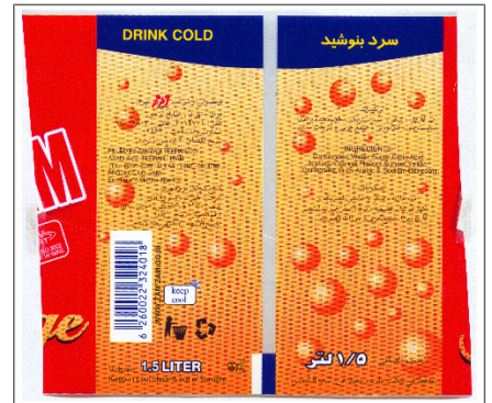
Fig. 92: More than one colour in the scanning area before and after the register mark and minimum size of the scanning area not considered
