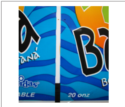
Fig. 90: More than one colour in the scanning area before and after the register mark and colour contrast not sufficient
