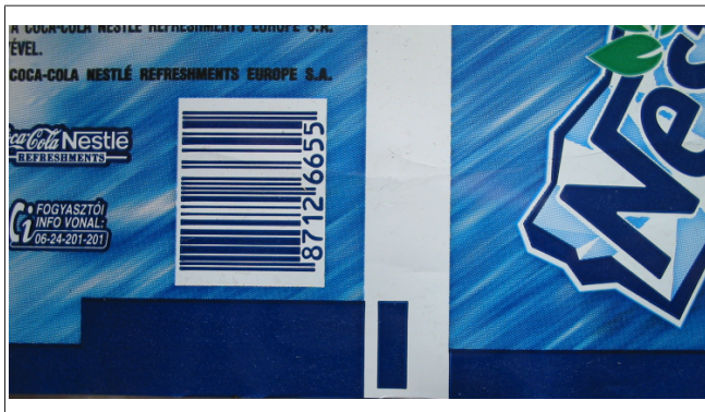
Fig. 93: More than one colour in the scanning area before and after the register mark
