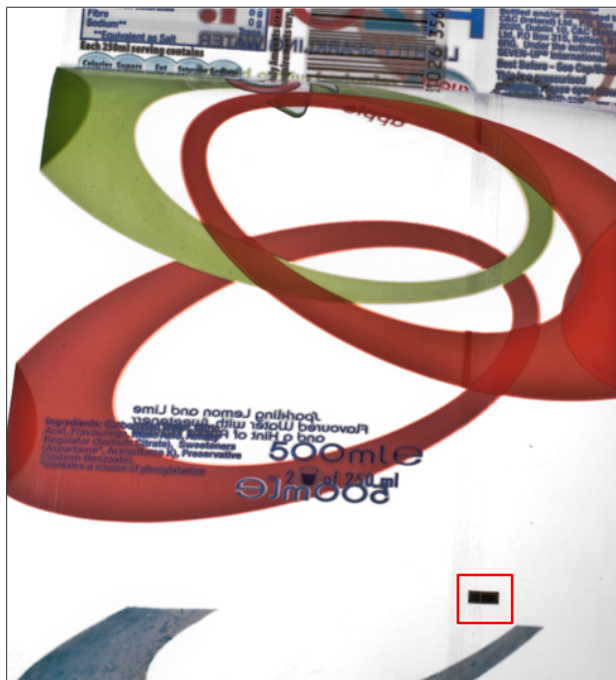
Fig. 120: Readable colour contrast register mark
