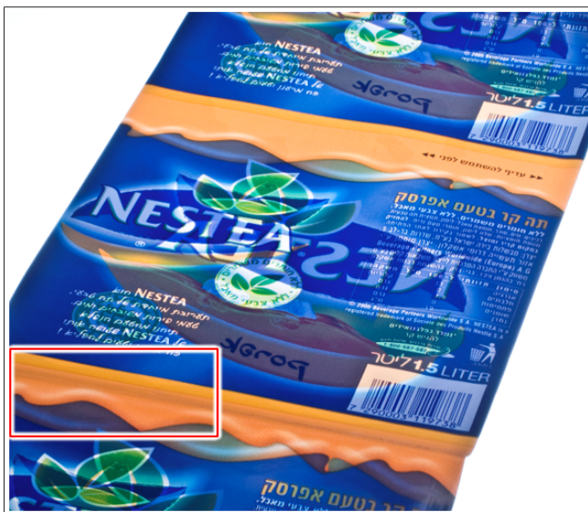
Fig. 116: Readable luminescent register mark
