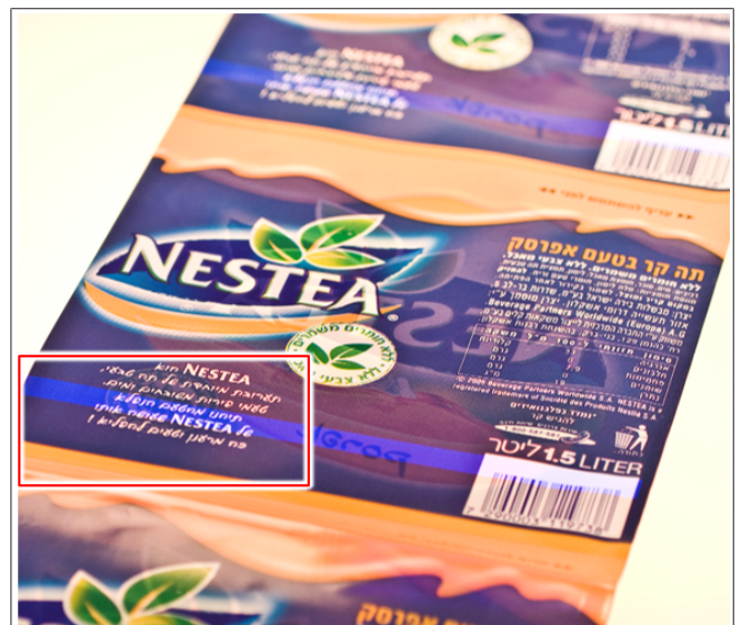
Fig. 117: Readable luminescent register mark
